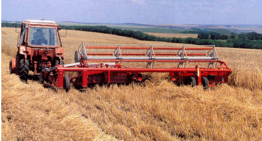
Fig. 1. Asymmetric swath header ZVP-6 machine-and-tractor aggregate during field experimental research
